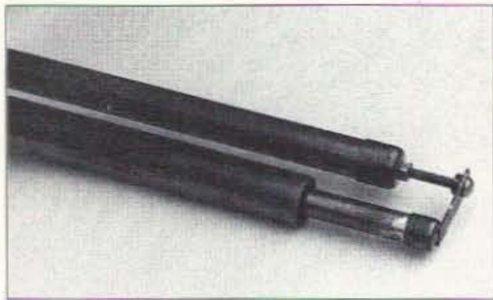
Photo C. Close-up of the tuning assembly of the coaxial capacitor.
